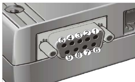
Figure 4: EIS/RS-232 interface (D-Sub 9-pole)
